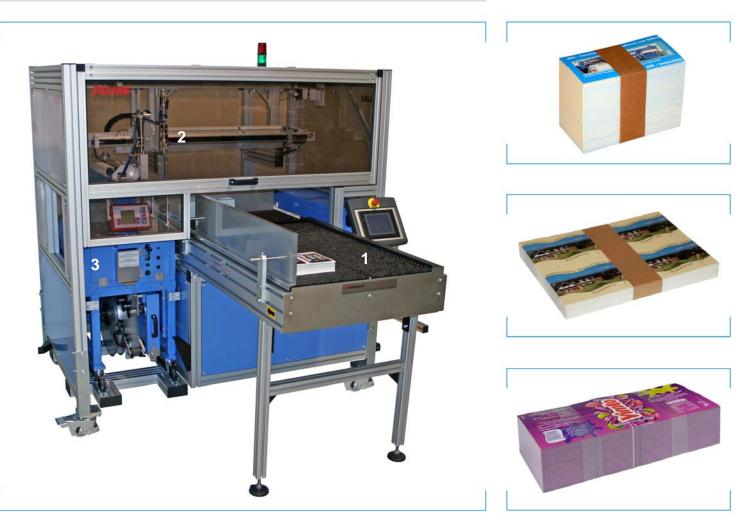
Cutter operator(s) load stacks of varying size onto the in-feed conveyor (1). Each stack is pushed and simultaneously measured by the servo driven linear pusher (2) into the banding machine (3). Banded stacks are discharged and ready for conveyance or easy handling.
