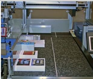
Stacks of varying height, width, and length can be processed back-to-back automatically without the need to make any adjustments to the machine.
